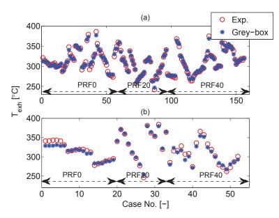
**Figure 3.13:** Prediction of  $T_{exh}$  (exhaust gas temperature) for Ricardo engine: (a) training, (b) validation data [1,2].
