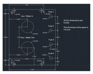
(a) Interface panel for fuel and water lines 2D design
