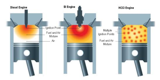
Figure 1.1: HCCI engine versus traditional engines [19].
