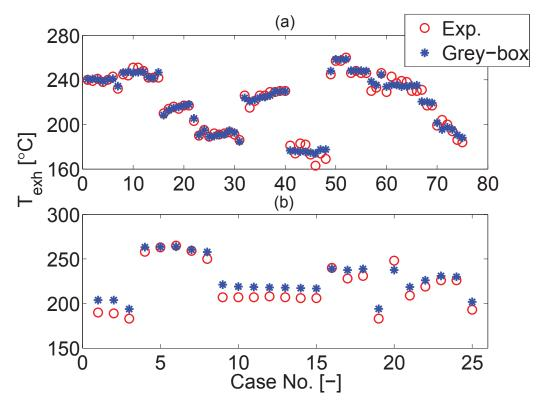
**Figure 3.21:** Prediction of  $T_{exh}$  for <u>Yanmar engine</u>: (a) Training, (b) Validation [1,2].
