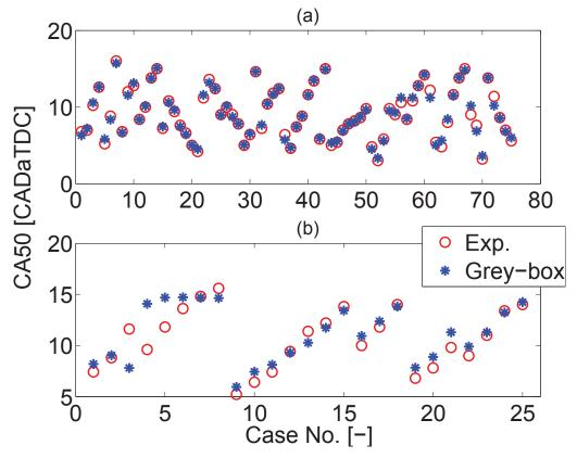
**Figure 3.19:** Prediction of CA50 for <u>Yanmar engine</u>: (a) Training, (b) Validation [1,2].
