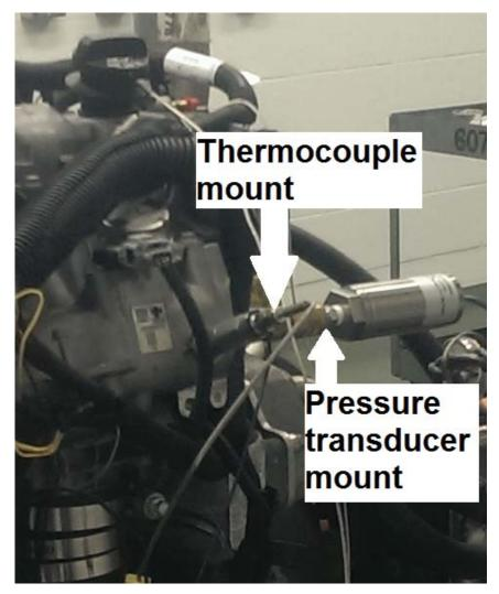
**Figure 2.14:** Pressure transducer and thermocouple on the intake manifold (photo by author).
