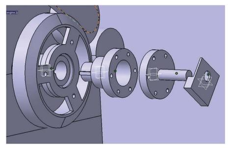
Figure 2.16: Exploded view of encoder mount 3D design.
