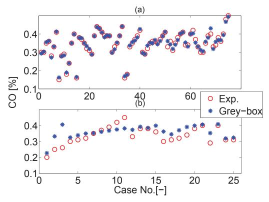
**Figure 3.22:** Prediction of CO for <u>Yanmar engine</u>: (a) Training, (b) Validation [1,2].
