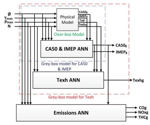
Figure 3.5: Architecture of the grey-box HCCI model [1,2].
