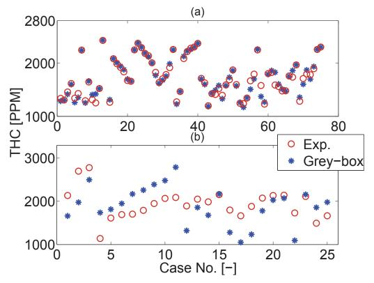
**Figure 3.23:** Prediction of THC concentration for <u>Yanmar engine</u>: (a) Training, (b) Validation [1,2].
