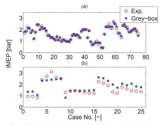
**Figure 3.20:** Prediction of IMEP for <u>Yanmar engine</u>: (a) Training, (b) Validation [1,2].
