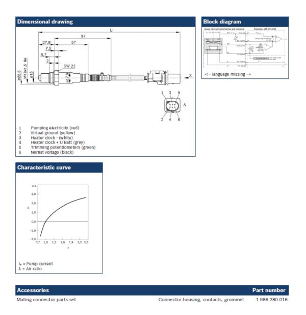
Figure C.9: Technical data 3 of lambda sensor.
