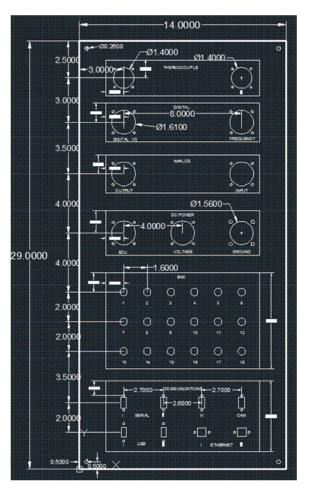
(**b**) Interface panel electrical connections 2D design
