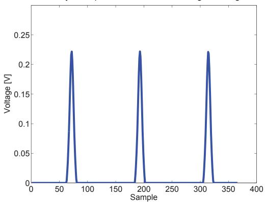
In-cylinder pressure transducer voltage reading
