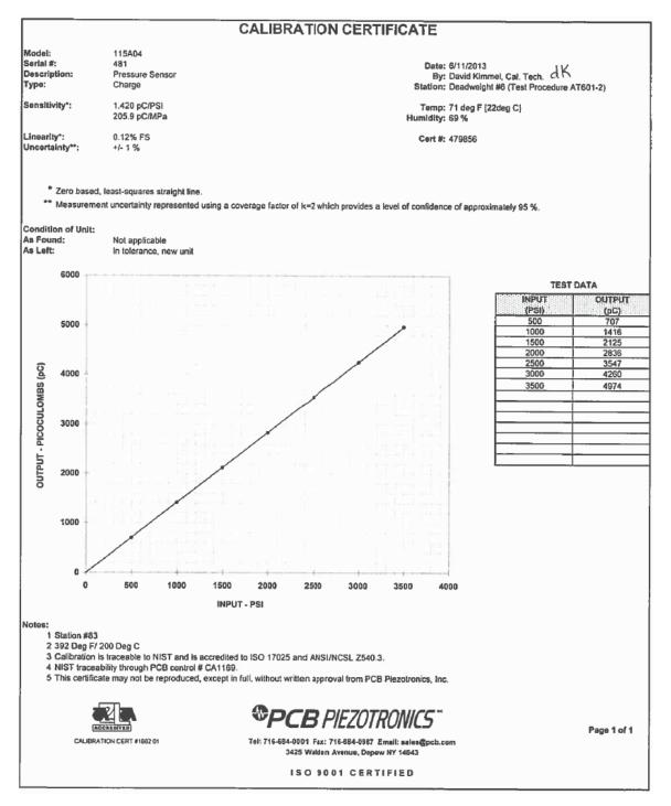
Figure C.2: Technical data sheet 2 of incylinder pressure transducer
