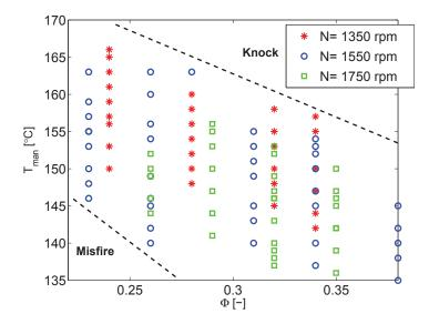
**Figure 3.18:** Operating range for the HCCI experimental data from Yanmar engine [1,2].
