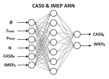
**Figure 3.6:** Feedfoward Artificial Neural Networks (ANN) for CA50 and IMEP used in this study [1,2].
