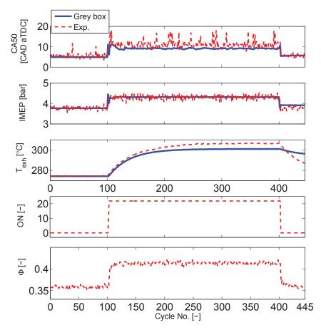
**Figure 3.17:** Validation of the CA50-IMEP,  $T_{exh}$  grey-box models for transient fueling conditions in Ricardo engine ( $P_m$ = 110 kPa,  $T_m$ = 91 C, External EGR = 0%,  $P_{exh}$ = 99 kPa, N=815 rpm) [1,2].
