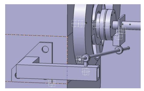
Figure 2.17: Encoder mount 3D design.
